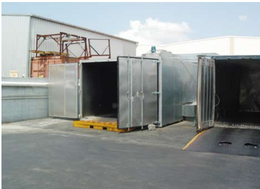
Modified containers (Kilquick, Brisbane) used for heat treatment to ISPM No. 15 (J. Banks)
