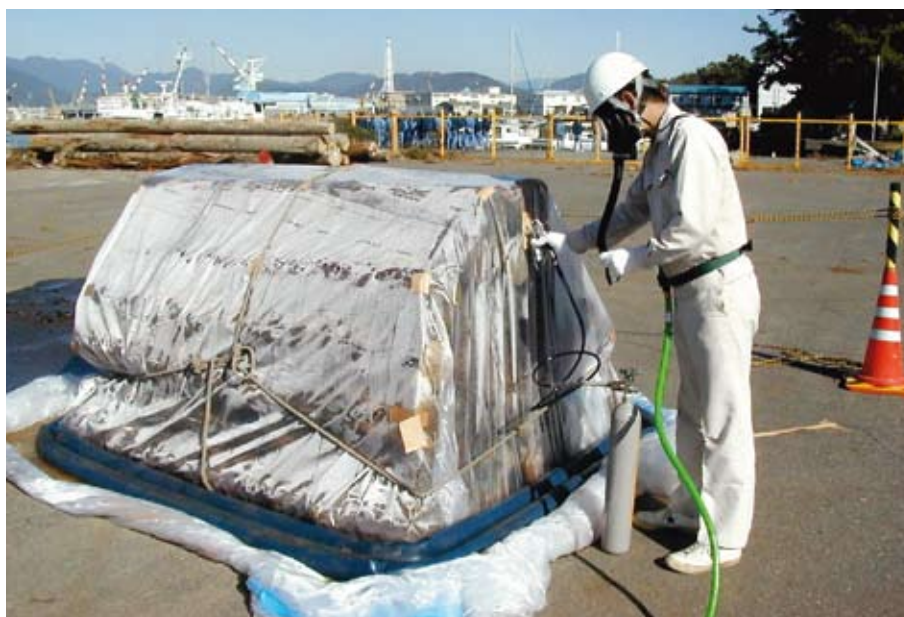
Experimental application of a methyl bromide alternative (sulphuryl fluoride/methyl isothiocyanate mixture) to timber, potentially for ISPM No. 15 (Ministry of Agriculture, Forestry and Fisheries, Japan)
