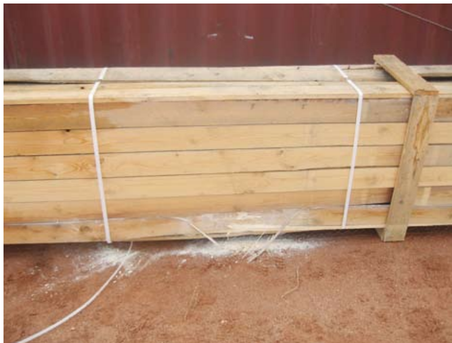
Damage to timber packaging material, showing presence of quarantine pests at import. Treatment with methyl bromide or alternatives required (AQIS, Australia)
